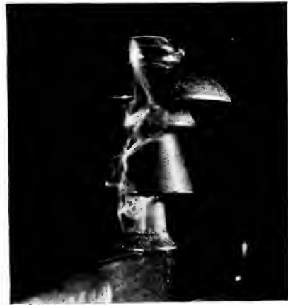
FIG. 14.—INSULATOR UNDER TEST AT 75,000 VOLTS.
